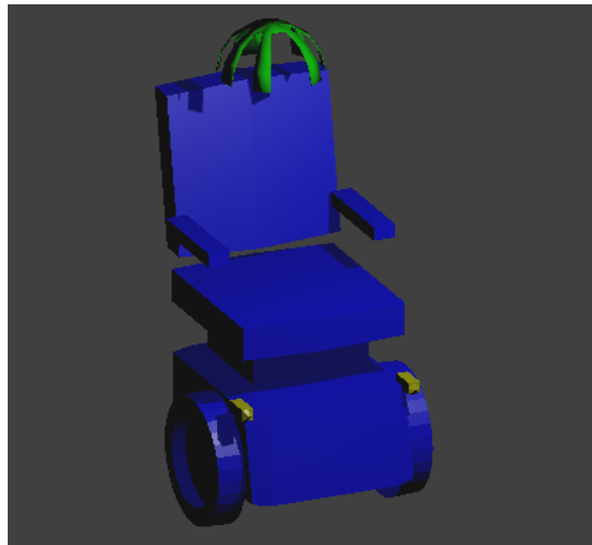
Figure 1: Wheelchair (blue) with BCI (green) and example sensor placement (yellow)
